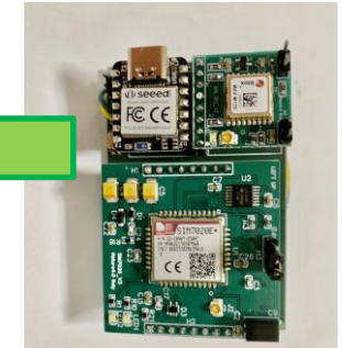
Environmental temperature and humidity + GPS + movement
